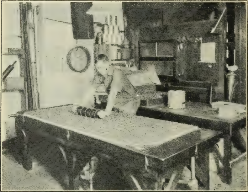
FIG. 33.—Cutting peanut candy into 5-cent bars. As the candy hardens quickly, the cutting must immediately follow the rolling to a uniform thickness seen in Figure 32
